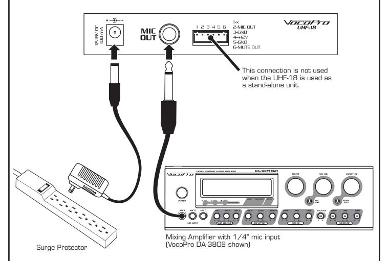
NOTE: Use the power adapter only when using the UHF-18 as a stand alone unit as shown above. Connecting the power adapter when using the UHF-18 as a plug-in module may result in damage to the UHF-18.
