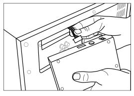
5. Carefully slide the UHF-18 into the expansion port, and secure it in place using the two screws.
