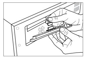
4. Attach the connection cable to the UHF-18. **NOTE**: The 1/4" jack and DC power input are not used when the UHF-18 is used as a plug-in module.
