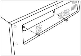
3. Pull the expansion port cover from the expansion port, and disconnect the connection cable.
