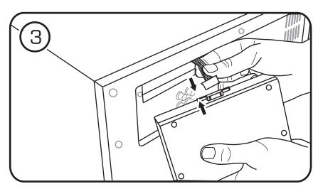
Firmly connect the cable to the plug on the back of the VHF-MODULE.
