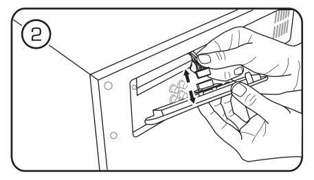
Carefully remove the cable from the plastic cover. **NOTE:** Be sure that the cable does not fall back into the unit. It may be necessary to temporarily secure the cable to the unit with a small piece of tape to prevent it from falling back into the unit.
