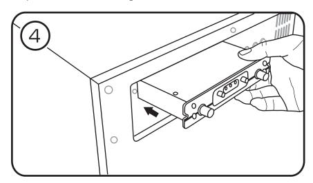
Slide the VHF-MODULE into the expansion slot, and secure it with the two screws.
